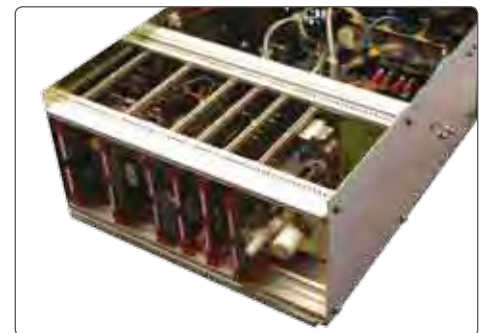
The modular design of Quark CPET minimizes technical assistance by means of boards replacement.
