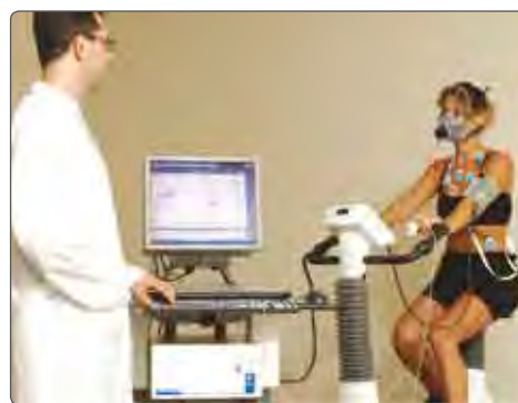
The CPET module add the possibility of performing pulmonary gas exchange analysis during exercise.
