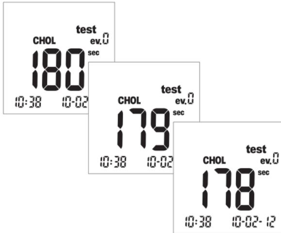
The time needed to evaluate the sample varies depending on the test parameter. This time is shown in the display and counted down to "0." The measurement times of the individual test parameters are:
