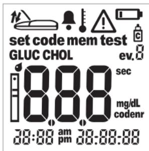
Every time the instrument is powered on, you should check the display. The instrument temporarily shows all symbols that may appear in the display.
