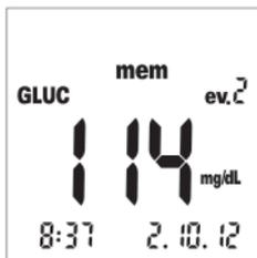
After the usual display test has been performed when switching on the instrument, the last stored measured value is displayed.
