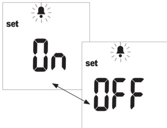
**11** Press the **M** button to switch between *OFF* and *On* (default setting).
