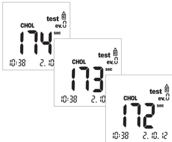
The measurement time varies depending on the test parameter. This time is shown in the display and counted down to "0." The measurement times of the individual test parameters are:
