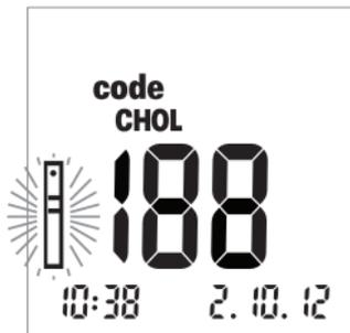
The three-digit code number (which is also printed on the reverse side of the code strip and on the test strip container) is shown in the display.
