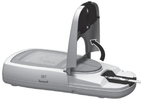
A flashing arrow now instructs you to open the measurement chamber flap to apply the blood. Explanations on flagging this measurement (events, *ev. 0* display or control flag) are provided later in this chapter.
